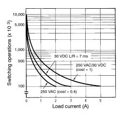
A maximum current of 0.15 A can be switched at 125 VDC (cosf = 1) and a maximum current of 0.1 A can be switched if L/R is 7 ms. In either case, a service life of 100,000 operations can be expected. The minimum applicable load is 10 mA at 5 VDC (failure level: P).
