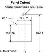
**Note:** Recommended mounting panel thickness: 1 to 3.2 mm.
